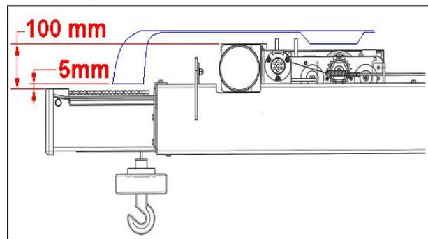
3.1.3.2 The door opening must at least be located 95 mm below and the roof profile must be located on the inside side (distance of the top side of the inner lifting arm and winch 100 mm minus the previously mentioned clearance of 5 mm); see the above sketch.
