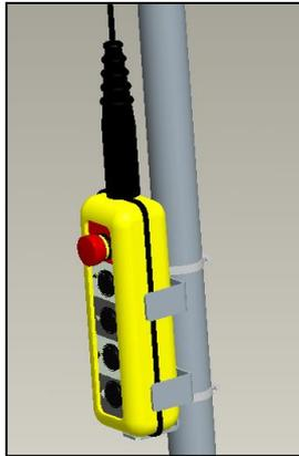
The handheld unit can be kept in the bracket for this purpose. The bracket should be installed on the post of the rear frame by using the two pipe clamps. The location can be freely selected by the end user. The connecting cable is sufficiently long to fasten the support for the handheld unit on both the left and the right post even when asymmetrically installing the EasyLoad.
