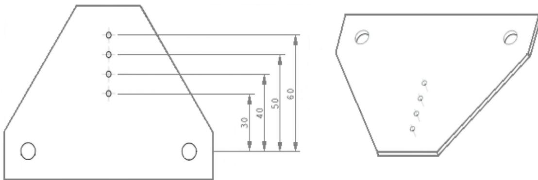
3.2.2 **130 triangular plate:** distance from the frame to the roof member varies from between 70 and 100 mm.
