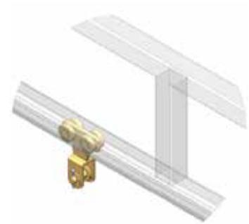
Figure 24: Installation of trolleys
