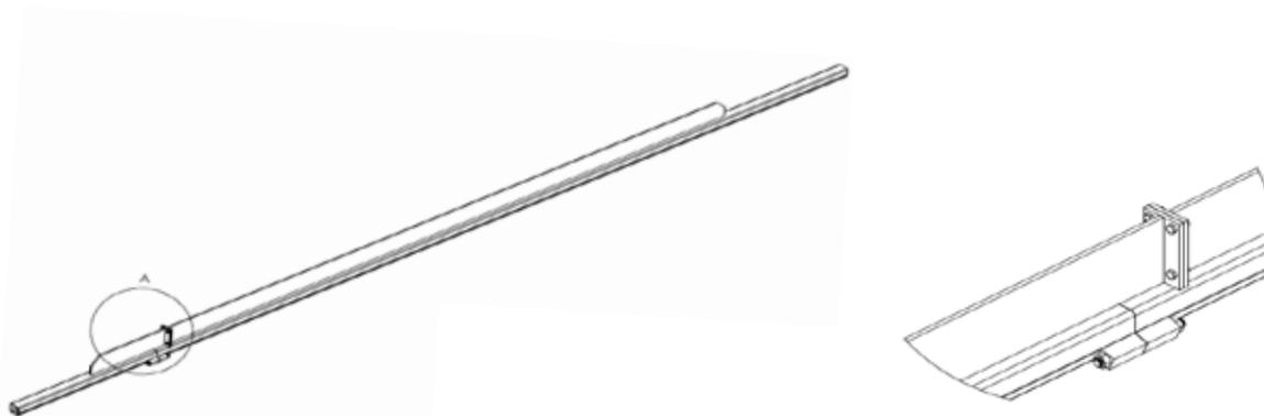
Figure 14: Junction using special plate and chocks
